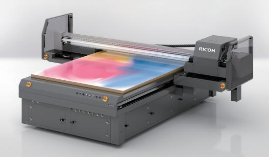
The new RICOH Pro T7210 UV flatbed is the ideal platform when printing onto a wide range of substrates requiring flexible ink with excellent adhesive properties. Productivity is further enhanced with the integrated vacuum table with pin registration that allows easy positioning of materials that are held firmly in place whilst printing. Full bleed printing eliminates the need for unnecessary trimming further reducing the time to dispatch the finished job.
